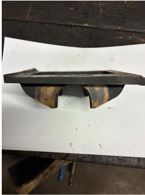
Fig.13 The worn HP slide valve kept under the workbench.
